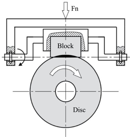
The samples were tested using a computer-aided block-on-disc sliding wear-testing machine with the contact pair geometry in accordance with ASTM G 77–83. A schematic configuration of the test machine is shown in Fig. 1. More detailed description of the tribometer is available elsewhere<sup>15,16</sup>.
