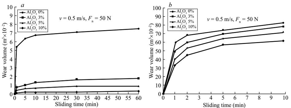
**Fig. 3.** Wear curves of tested materials: lubricated sliding (a), dry sliding (b)
