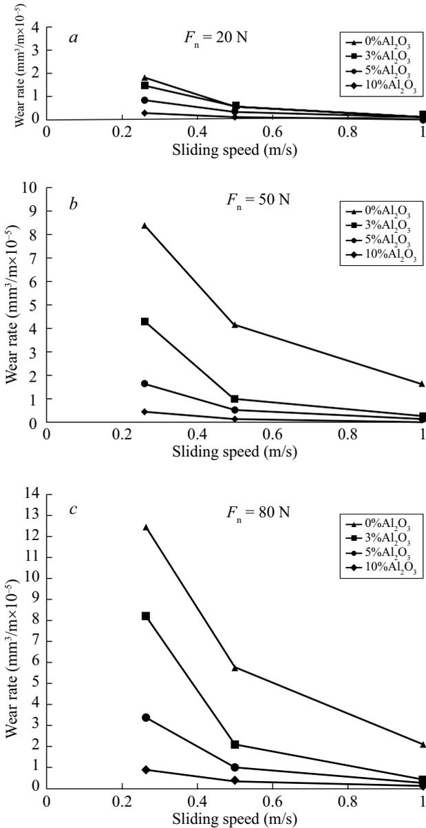
The incorporation of  $Al_2O_3$  particles to the ZA-27 alloy improves the sliding wear resistance in comparison with the unreinforced alloy. The effects of both applied speed and load, during lubricated and dry sliding were investigated as a function of  $Al_2O_3$  wt. %.
