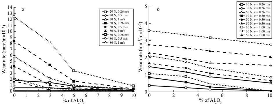
Fig. 6. Wear rate versus wt. % of  $\text{Al}_2\text{O}_3$ : lubricated sliding (a), dry sliding (b)
