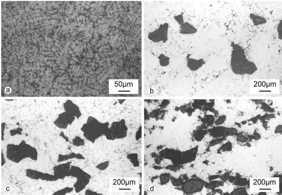
**Fig. 2.** Microstructure of the tested materials: ZA-27 alloy (a), composite 3%  $\text{Al}_2\text{O}_3$  (b), composite 5%  $\text{Al}_2\text{O}_3$  (c) and composite 10%  $\text{Al}_2\text{O}_3$  (d)
